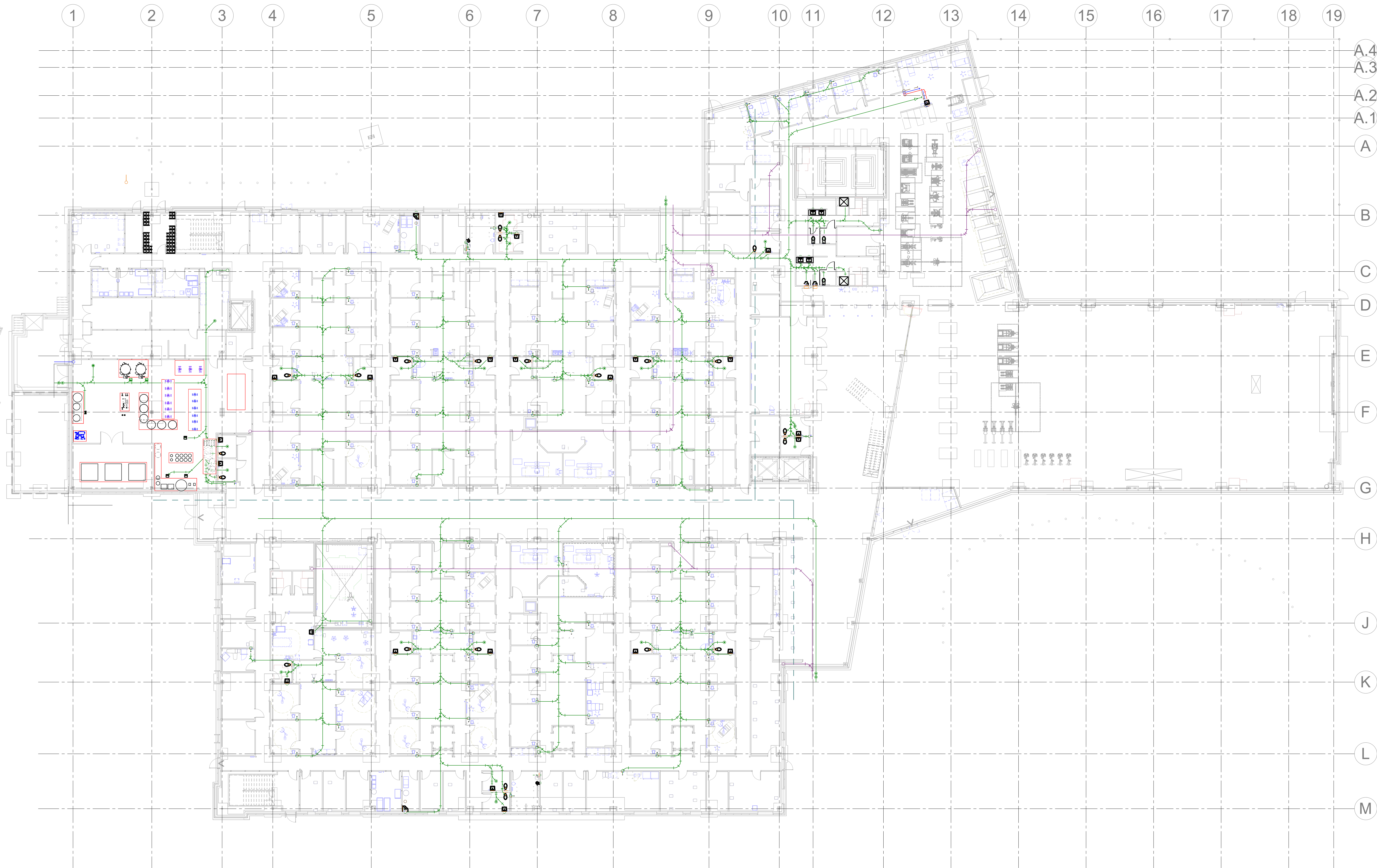
1 LEVEL 1 PLUMBING UNDERFLOOR PLAN 1/16" = 1'-0"
